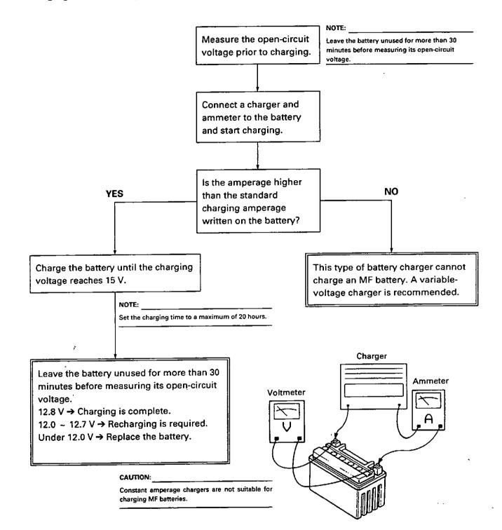
CHECKING AND CHARGING THE BATTERY/ CHECKING THE FUSES
