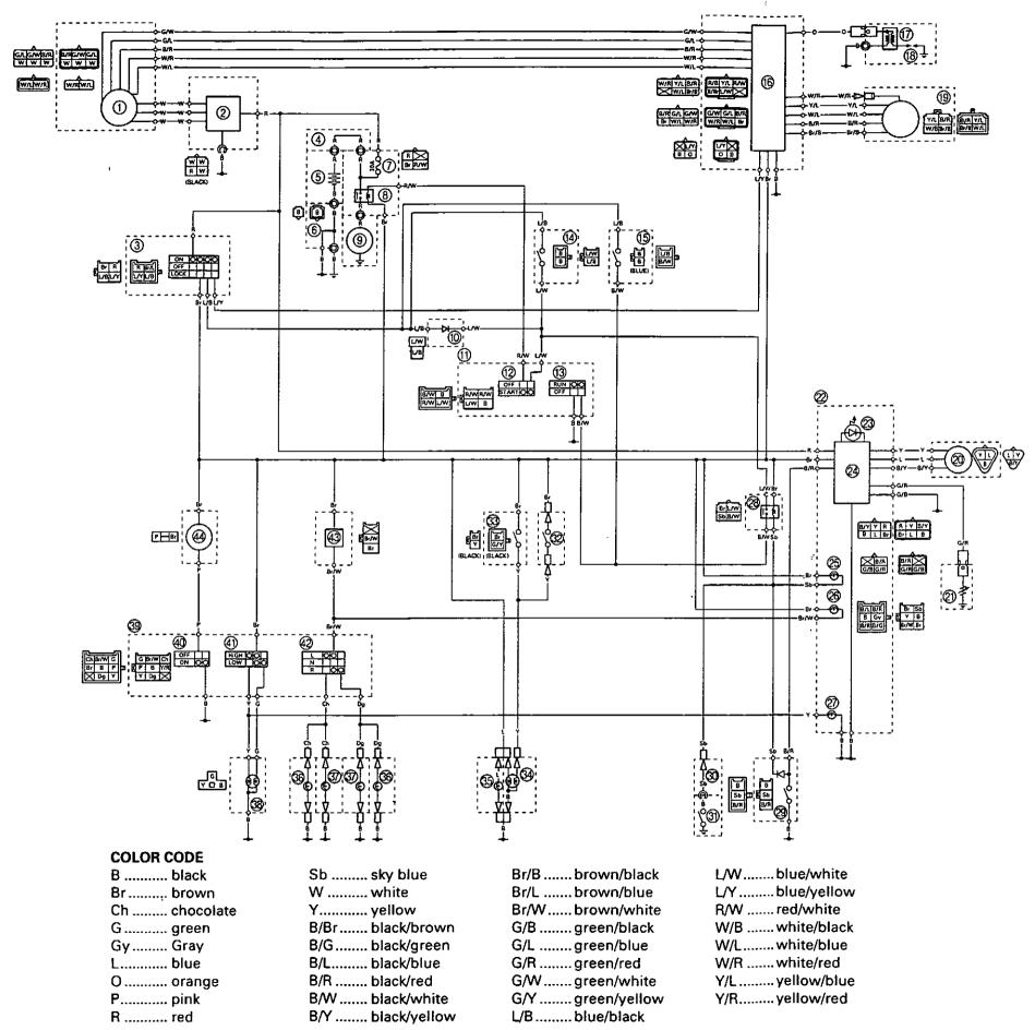
① CDI magneto ② Rectifier/regulator ③ Main switch (4) Battery positive lead **(5)** Battery 6 Battery negative lead ⑦ Main fuse (8) Starter relay (9) Starter motor 10 Diode (1) Right handlebar switch 12 Start switch Brine stop switch (i) Clutch switch (5) Sidestand switch 6 CDI unit 🗑 Ignition coil (B) Spark plug
