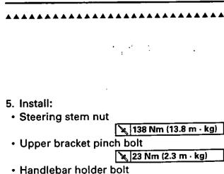
landlebar holder bolt 🔀 23 Nm (2.3 m · kg)
