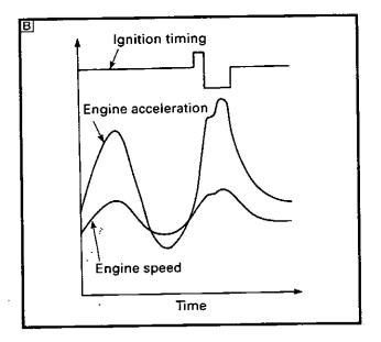
3. Comparison of ignition timing with and without traction control
