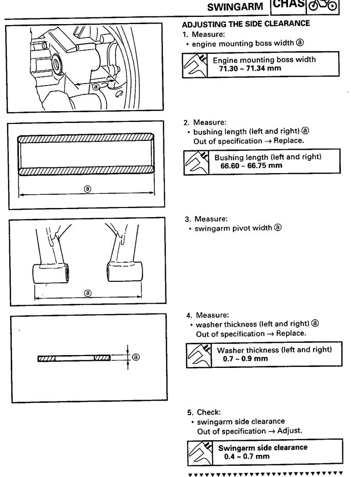
a. Calculate the swingarm side clearance by using the formula given below.
