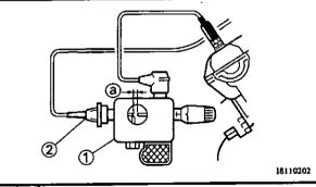
Minimum ignition spark gap 6 mm
