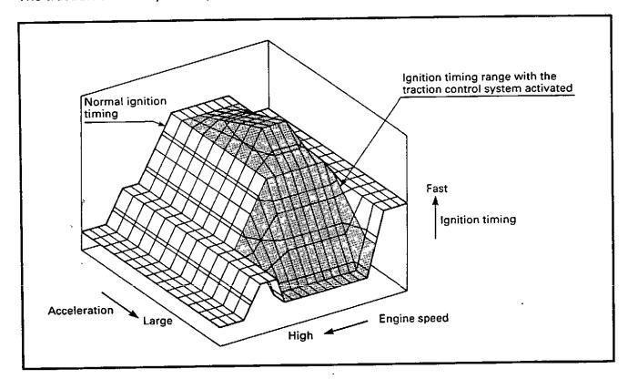
The traction control system operates at engine speeds between 3,000 and 8,000 r/min.
