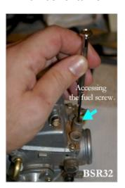
3. Turn the fuel screw counterclockwise ¼ turn past the number of turns counted in step # 2 (if this results in turning it out 2 turns past stock {see the chapter taking stock of your bike}, you should replace the pilot jet with a larger one and start again with the fuel screw at one turn out)
