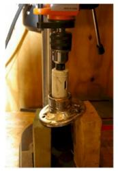
Use plenty of oil when drilling. After removal, it will be necessary to file down the rough edges produced by drilling. It will also be necessary to remove any metal shavings that might have fallen into the spark arrestor. Use compressed air to carefully blow these out.
