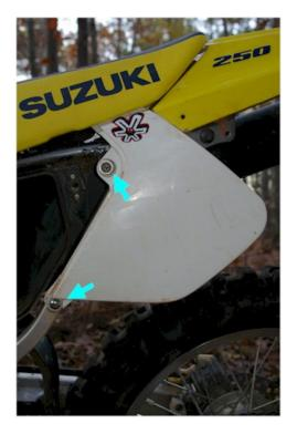
Next, remove the seat by unscrewing the two seat retaining bolts, and lift the seat off.
