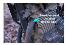
Place the header in a vise and using the half-round file, begin to file the weld down until it is flush with the pipe. Power tools may be substituted if available.
