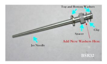
Remove washers and spacers, and insert 1 (one) .025" washer where indicated above. Reassemble.
