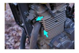
Loosen the oil cooler for clearance
