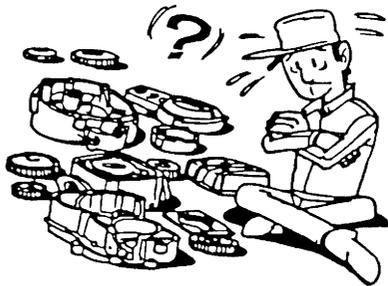
4. During disassembly, clean all of the parts and place them in trays in the order of disassembly. This will speed up assembly and allow for the correct installation of all parts.
