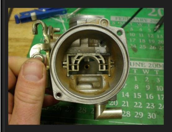
2- check that your cap-sealing surface is flat. (there have been some people who have found that their cap became warped due to the stupid 2 bolt design. this allowed even more dirt to enter the carb and started causing problems.) to check if it is flat, find any level straight surface (small piece of glass is the best) and check. you can also use a straight edge to check for flatness as well. If you find your cap is warped, sorry but ya gotta buy a new one....
