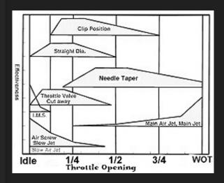
air screw = 0 - 1/8 throttle pilot jet = 1/8 - 1/4 throttle slide valve = 1/8 - 1/2 throttle needle = 1/4 - 3/4 throttle main jet = 3/4 - 1/8 full throttle
